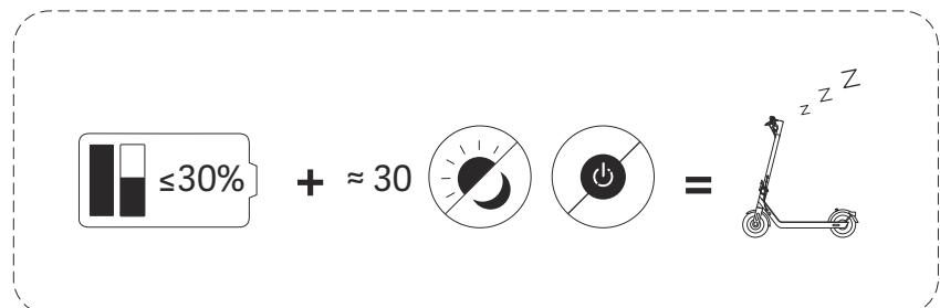
When the scooter is turned off for about a month with the battery level of the scooter being lower than 30%, the scooter will enter sleep mode. In this case, the scooter cannot be turned on. To exit the sleep mode, charge the scooter for about three seconds to activate the battery.
